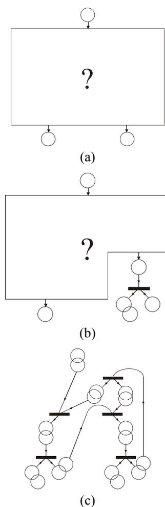
Figure 7. Steps of the synthesis method: (a) problem definition; (b) subproblem generation in the first step; and (c) resultant final structure.
