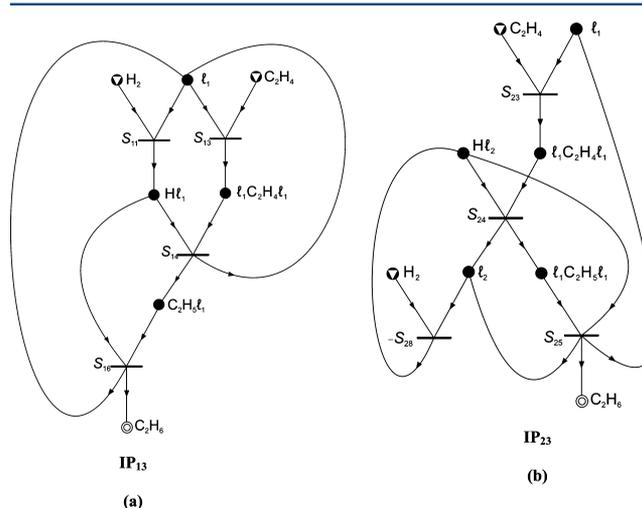
**Figure 3.** P-graph representations of feasible independent pathways based on: (a) the biactive-site mechanism,  $\text{IP}_{13}$ , and (b) the triactive-site mechanism,  $\text{IP}_{23}$ .
