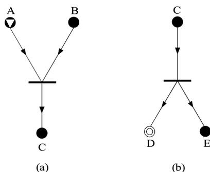
**Figure 1.** P-graphs of some operating units and their concomitant material streams: (a) Materials A, B, and C, and operating unit ( $\{A, B\}$ ,  $\{C\}$ ) and (b) Materials C, D, and E, and operating unit ( $\{C\}$ ,  $\{D, E\}$ ).
