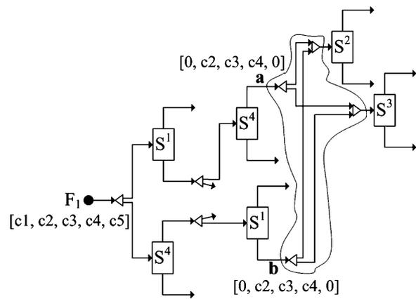
Fig. 6. Part of the super-structure after merging separators.
