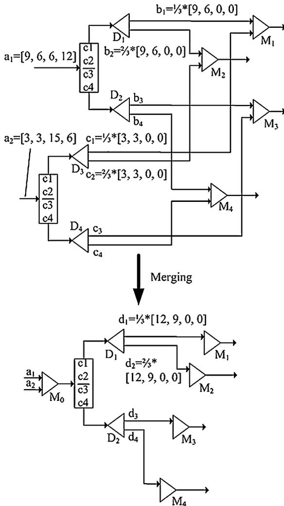
Fig. 3. Merging of separators with the identical splitting ratios.
