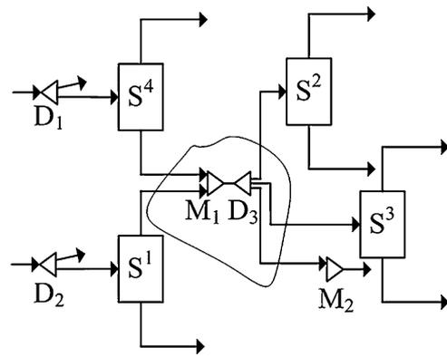
Fig. 13. Material balance around a mixer–divider pair.
