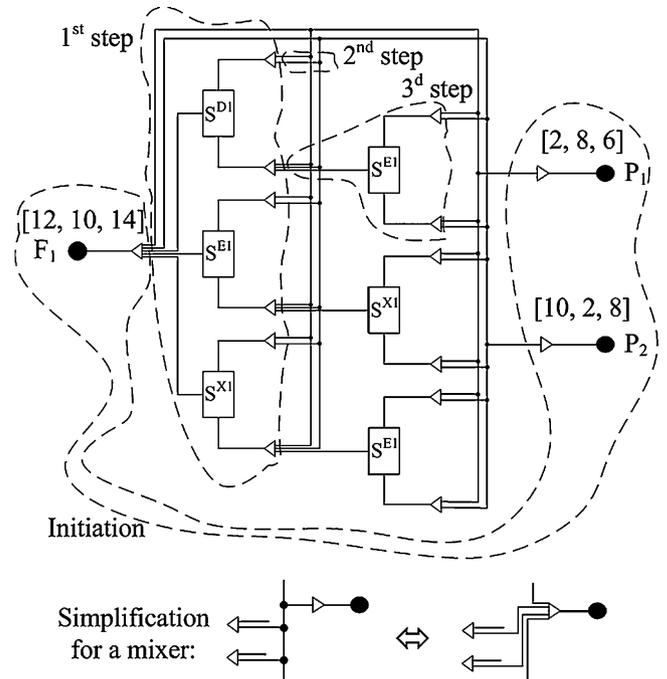
Fig. 2. Step-by-step generation of the unreduced super-structure: for clarity, every mixer in this and all other figures is simplified as illustrated.
