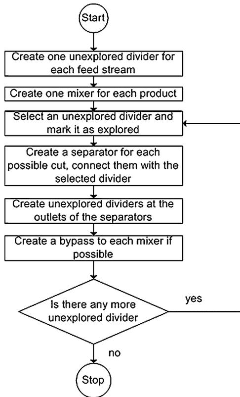
Fig. 1. Flowchart for generating the unreduced super-structure.
