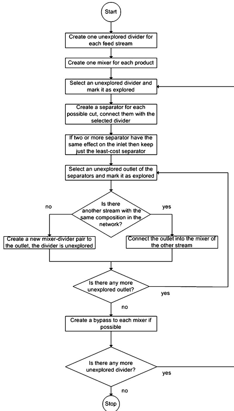
Fig. 8. Flowchart for generating the reduced super-structure.
