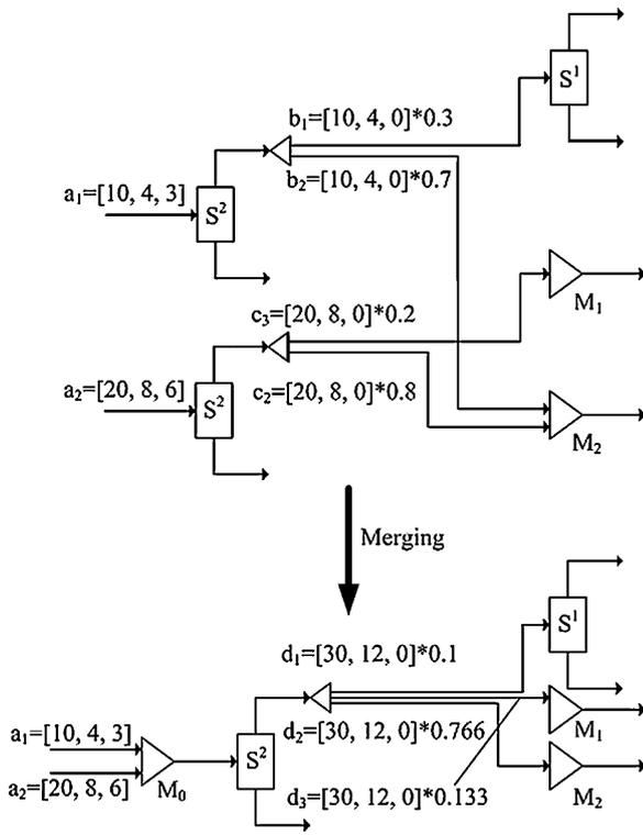
Fig. 4. Merging of separators with identical inlet composition.
