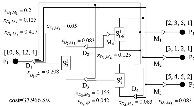
Fig. 14. Optimal structure of the first example.
