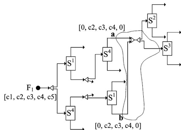
Fig. 7. Part of the super-structure after exchanging the positions of dividers and mixers.
