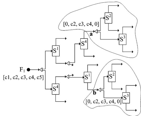
Fig. 5. Part of the super-structure before merging separators.
